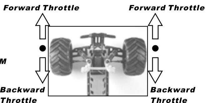
Throttle Trim is always applied to set and adjust the idle speed of your car.
