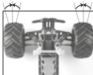
Place your car on the stand with wheels off the ground, and then tune the steering trim to align the front wheels.
