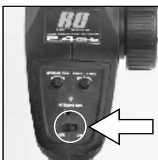
Switch off the ESC/Receiver switch as shown in the picture. Switch off the power switch on the radio controller.
