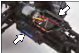
Open the battery compartment and remove the batteries from the car. Use Only the provided charger and charger box to charge the batteries for your car. Connect the charger box with the charger, and load the batteries onto the charger box. Always observe correct polarity (plus/+ and minus/-) . The polarity is indicated in the charger box.
