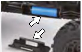
Open the battery compartment and remove the batteries from the car.
