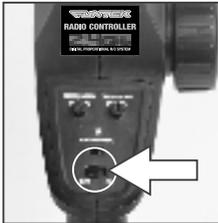
Switch on the power switch on the radio controller.
